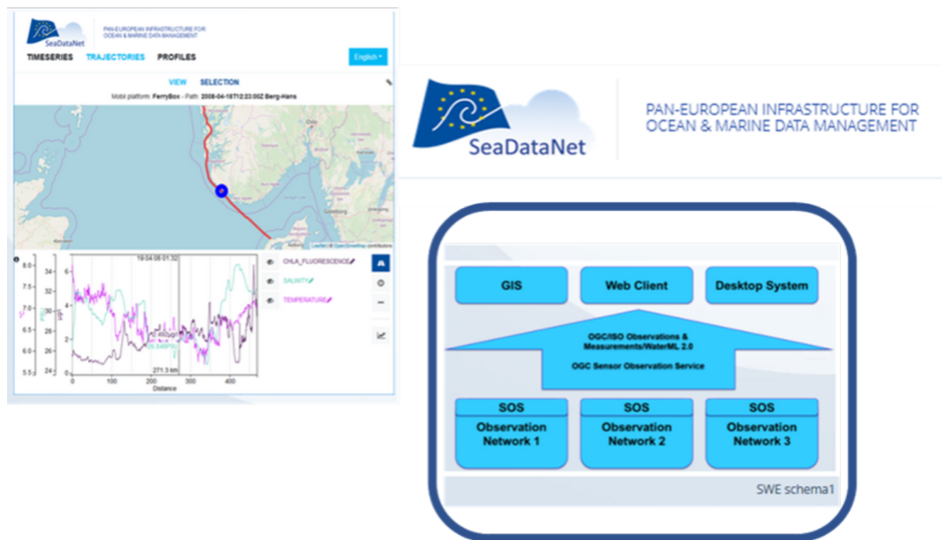
Figure 4.5 SeaDataNet employs OGC Sensor Web standards to ease access, ingest and viewing of observations from a range of fixed and mobile sensor assets
